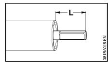
The drive shaft must not project from the tube more than L = 22 mm (7/8 in).
