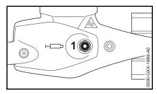
Check the lubricant level at regular intervals of about every 25 hours of operation. Unscrew the filler
